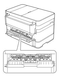
17 Close the inside cover and Jam Clear Cover. Make sure the covers are closed completely.
