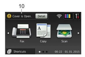
The warning icon ! appears when there is an error or maintenance message; press Detail to view it, and then press
