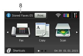
When Fax Preview is set to Off, Stored Faxes displays how many received faxes are in the machine's memory.
