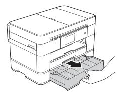
Push the blue slider until it locks in the release position, and then extend the tray until the blue slider returns to and locks in the default position. Make sure the triangular mark inside the tray (1) lines up with the mark (2) for **B4 JIS/LGL**, as shown in the illustration.
