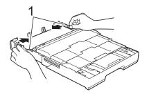
7 Check that the paper is flat in the tray and below the maximum paper mark (1). Overfilling the paper tray may cause paper jams.
