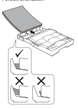
6 Gently adjust the paper guides (1) to fit the paper. Make sure the paper guides touch the sides of the paper.
