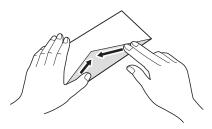
4 Load *only one* envelope in the manual feed slot with the printing surface **face up**.
