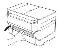
Pull out the paper support (1) until it locks into place, and then unfold the paper support flap (2).
