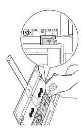
5 Fan the stack of paper well to avoid paper jams and misfeeds.
