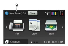
When Fax Preview is set to On, New Fax(es) displays how many new faxes you have received and stored in the machine's memory.
