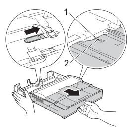
Push the blue slider a second time until it locks in the release position, and then extend the tray until the blue slider returns to and locks in the default position. Open the tray cover and make sure the triangular mark inside the tray (1) lines up with the mark (2) for **A3/LGR**, as shown in the illustration.
