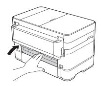
9 Using both hands, use the finger holds on each side of the machine to lift the scanner cover (1) into the open position.
