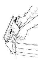
6 Put one envelope in the manual feed slot until the front edge touches the paper feed roller. Let go of the envelope when you hear the machine pull it in a short distance. The Touchscreen displays Manual Feed Slot ready.
