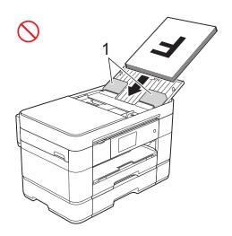
If you load a small size document and cannot remove it, open the stack tray (1) and then remove the document.
