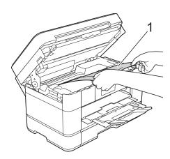
Move the print head (if necessary) to reach any paper remaining in this area. Make sure no jammed paper is left in the corners of the machine (1) and (2).
