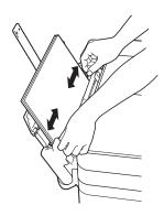
8 Pull out the paper support (1) until it locks into place, and then unfold the paper support flap (2).
