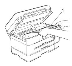
Move the print head (if necessary) to reach any paper remaining in this area. Make sure no jammed paper is left in the corners of the machine (1) and (2).
