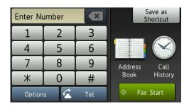
To change the fax-sending settings, press Options. Swipe up or down or press ▲ or ▼ to scroll through the fax settings. When the setting you want is displayed, press it and choose your new option. When finished changing options, press OK.
