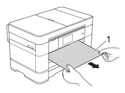
5 Lift the Jam Clear Flap, and remove the jammed paper.
