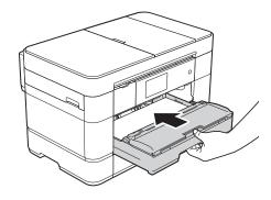
8 Pull out the paper support (1) until it locks into place, and then unfold the paper support flap (2).
