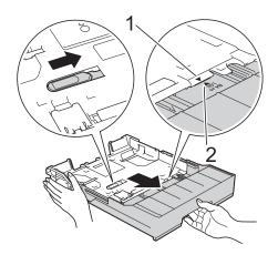
Push the blue slider a second time until it locks in the release position, and then extend the tray until the blue slider returns to and locks in the default position. Make sure the triangular mark inside the tray (1) lines up with the mark (2) for **A3/LGR**, as shown in the illustration.
