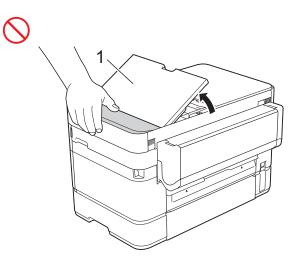
DO NOT carry the product by holding the scanner cover, the Jam Clear Cover, manual feed slot cover, MP tray or control panel. Doing so may cause the product to slip out of your hands.
