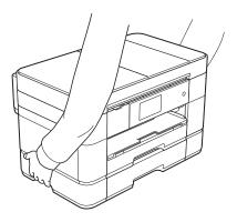
When carrying the product, remove the tray if it has been extended to hold large paper such as A3, Legal or ledger size paper. The weight of the paper could cause the tray to fall and cause injury to you.
