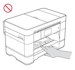
Do not apply weight or pressure to the gray shaded area shown in the illustration below. Doing so may cause the ADF document support (1) to inadvertently open.
