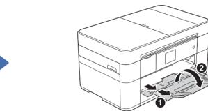
Pull out the paper support 1, and unfold the paper support flap 2.
