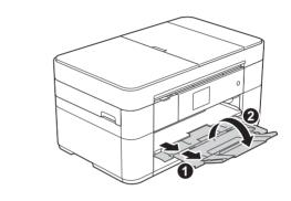
Pull out the paper support **1**, and unfold the paper support flap **2**.
