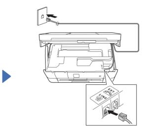
Connect the telephone line cord. Use the socket marked LINE and guide the cord out the back of the machine.
