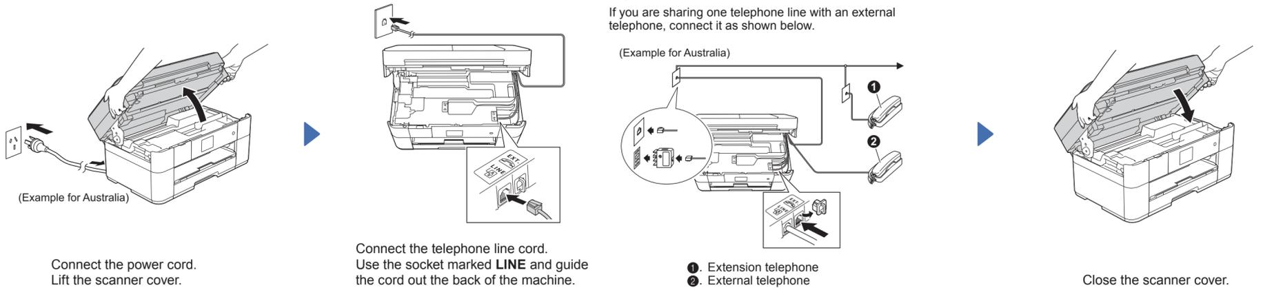
Connect the power cord. Lift the scanner cover.
