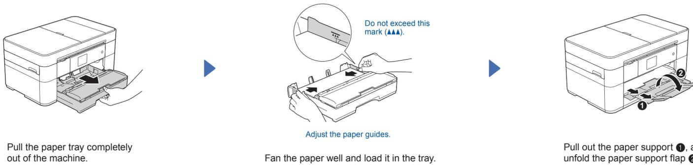
Pull the paper tray completely out of the machine.
