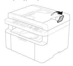
2 Load your document face down, top edge first in the ADF until the LCD message changes. 3 Adjust the paper guides (1) to fit the width of your document.
