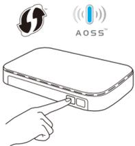
Press the WPS or AOSS™ button on your wireless LAN access point/router.
