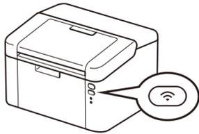
Press and hold the WiFi button on your machine for about 2 seconds. The WiFi button will light up when connected.
