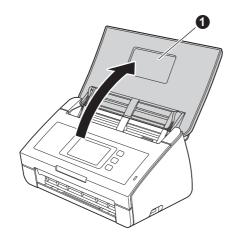
Pull the Output Tray out of the machine **1** and then unfold the Document Stopper **2**.
