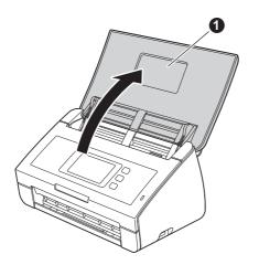
C Pull the Output Tray out of the machine **1** and then unfold the Document Stopper **2**.
