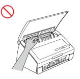
DO NOT carry the machine by holding the top cover. Doing this may cause the machine to slip out of your hands. Only carry the machine by placing your hands under the entire machine.
