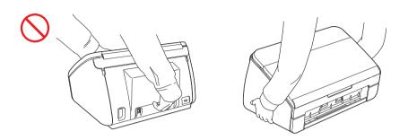
Use caution when operating the machine to prevent clothing (particularly sleeves, neckties, etc.), hair, or accessories from being drawn into the machine, otherwise injury may result. In the event that an object is drawn into the machine, immediately disconnect the machine from the power source.
