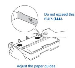
Fan the paper well and load it in the trav.
