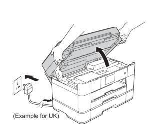
Connect the power cord. Lift the scanner cover.
