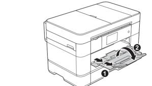
Pull out the paper support 1, and unfold the paper support flap 2.
