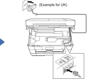
Connect the telephone line cord. Use the socket marked LINE and guide the cord out the back of the machine.
