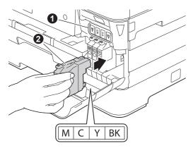
Gently push the back of the ink cartridge marked "PUSH" until the cartridge lever lifts. After all the ink cartridges are installed, close the ink cartridge cover.
