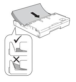
Gently adjust the paper side guides to fit the paper with both hands. Make sure that the paper side guides touch the sides of the paper.
