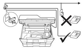
Set the receive mode to External TAD if you have an external answering machine. See Choose a Receive Mode on page 10. Detailed information ➤>Basic User's Guide: Connecting an external TAD (telephone answering device)
