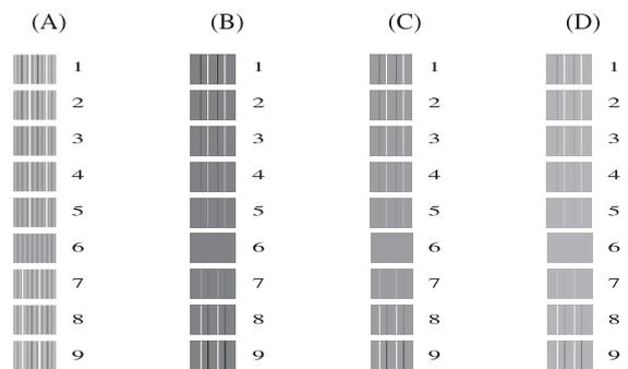
5 For the "A" pattern, swipe up or down, or press **▲** or **▼** to display the number of the test print that has the least visible vertical stripes (1-9), and then press it. Press **OK**.
