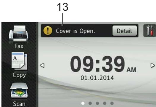
The warning icon
