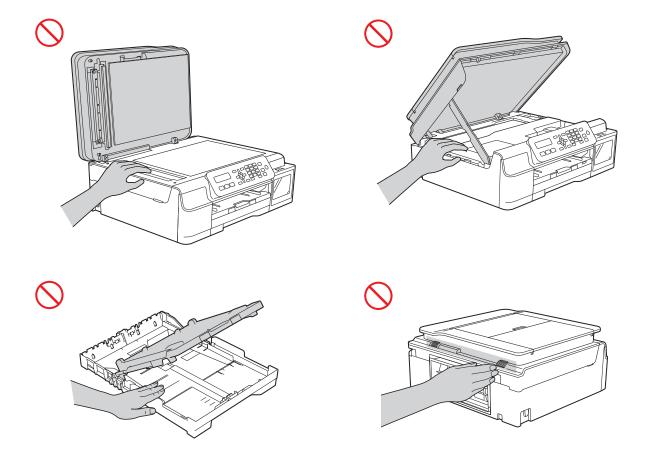
DO NOT carry the product by holding the scanner cover, the Jam Clear Cover or control panel. Doing so may cause the product to slip out of your hands.
