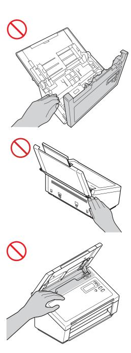
DO NOT carry the machine by holding the top cover. Doing this may cause the machine to slip out of your hands. Only carry the machine by placing your hands under the entire machine.
