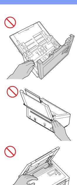
DO NOT carry the machine by holding the top cover. Doing this may cause the machine to slip out of your hands. Only carry the machine by placing your hands under the entire machine.
