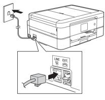
Connect the telephone line cord. Use the jack marked LINE and guide the cord out the back of the machine.
