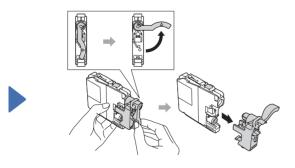
Follow the Touchscreen instructions to install the ink cartridges. The machine will prepare the ink tube system for printing.
