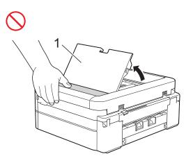
DO NOT carry the product by holding the scanner cover, the Jam Clear Cover, the manual feed slot cover (some models only), or the control panel. Doing so may cause the product to slip out of your hands.
