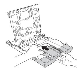
DO NOT touch the edges of the metal parts behind the rollers in the grey shaded area shown in the illustration. Doing this may cause injury to your fingers by cutting them.
