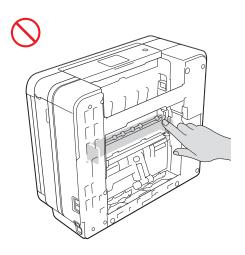
Do not apply pressure with your hand or elbow in the gray shaded area shown in the illustration below. Doing so may cause the ADF document support (1) to inadvertently open.
