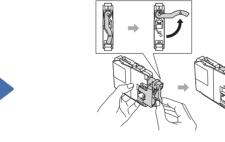
Follow the on-screen instructions to install the ink cartridges. The machine will prepare the ink tube system for printing.
