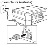
Connect the telephone line cord. Use the socket marked LINE.
