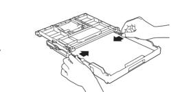
Fan the paper well and load it in the tray, and then adjust the paper guides.
