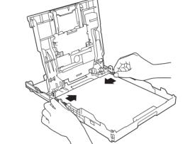
Fan the paper well and load it in the tray, and then adjust the paper guides.
