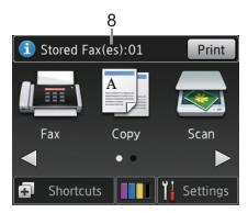
When [Fax Preview] <sup>1</sup> is set to [Off], [Stored Fax(es)] displays how many received faxes are in the machine's memory.
