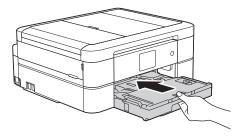
7. While holding the paper tray in the machine, pull out the paper support (1) until it locks into place, and then unfold the paper support flap (2).
