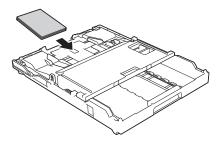
5. Gently adjust the paper width guides (1) to fit the paper. Make sure the paper width guides touch the edges of the paper and the paper is flat in the tray.
