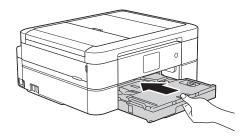
6. While holding the paper tray in the machine, pull out the paper support (1) until it locks into place, and then unfold the paper support flap (2).
