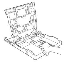
6. Close the output paper tray cover and put the paper tray firmly back in the machine.
