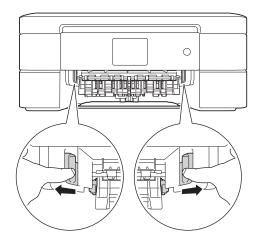
4. Place both hands under the plastic tabs on both sides of the machine to lift the scanner cover (1) into the open position.
