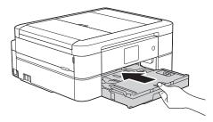
10. While holding the paper tray in the machine, pull out the paper support (1) until it locks into place, and then unfold the paper support flap (2).
