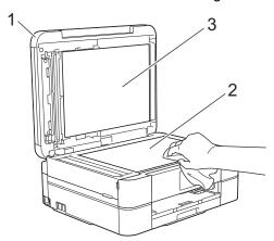
3. In the ADF unit, clean the white bar (1) and the glass strip (2) with a lint-free cloth moistened with a non-flammable glass cleaner. (ADF models only)
