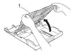
4. Gently press and slide the paper width guides (1) and then the paper length guide (2) to fit the paper size.
