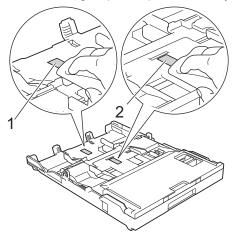
4. Clean the Paper Pick-up Rollers (1) with a soft lint-free cloth moistened with water. Slowly turn the rollers so that the whole surface is cleaned. After cleaning, wipe the rollers with a dry, soft lint-free cloth to remove all moisture.
