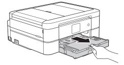
3. Press the blue photo paper tray release button (1) and slide whole the output paper tray cover forward until it locks into the photo printing position (2).
