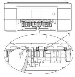
5. Lift the Jam Clear Flap (2), and then clean the back side of the Paper Feed Rollers (1) with a soft lint-free cloth moistened with water. After cleaning, wipe the rollers with a dry, soft lint-free cloth to remove all moisture.
