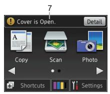
The warning icon ! appears when there is an error or maintenance message; press [Detail] to view it, and then press to return to Ready mode.
