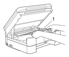
6. If the LCD displays [Repeat Jam A Inside/Front], move the print head (if needed) to take out any paper remaining in this area. Make sure scraps of paper are not left in the corners of the machine (1) and (2).
