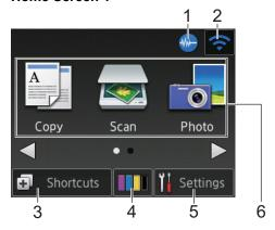
This screen shows the machine's status when the machine is idle. This Home screen is also called the Ready Mode screen. When displayed, this indicates that your machine is Ready for the next command.
