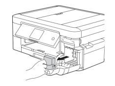
Open the ink cartridge cover, and then remove the orange protective part from the machine.
