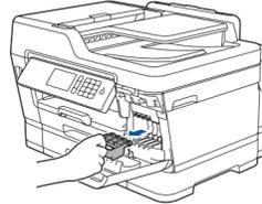
Open the ink cartridge cover and remove the orange protective part from the machine.
