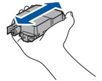
Quickly shake just the **black** ink cartridge horizontally 15 times as shown, before inserting it into the machine.
