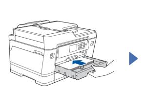
Slowly push the paper tray completely into the machine. Pull out the paper support until it locks into place.
