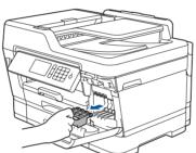
Follow the Touchscreen instructions to unpack and install the ink cartridges. The machine will prepare the ink tube system for printing.
