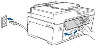
Connect the power cord. The machine will power on automatically.
