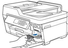
Open the ink cartridge cover and remove the orange protective part from the machine.
