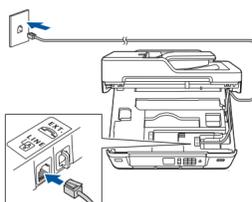
Connect the telephone line cord. Use the jack marked **LINE** and guide the cord out the back of the machine.
