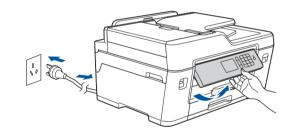
Connect the power cord. The machine will power on automatically.
