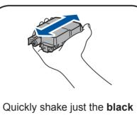
ink cartridge horizontally 15 times as shown, before inserting it into the machine.
