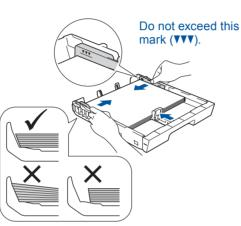
Adjust the paper guides. Load the paper in the tray with the printing surface down.
