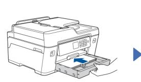
Slowly push the paper tray completely into the machine. Pull out the paper support until it locks into place.
