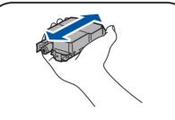
Quickly shake just the black ink cartridge horizontally 15 times as shown, before inserting it into the machine.
