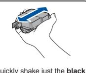
Quickly shake just the **black** ink cartridge horizontally 15 times as shown, before inserting it into the machine.
