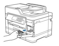
Open the ink cartridge cover, and then remove the orange protective part from the machine.
