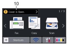
The warning icon \_\_\_\_ appears when there is an error or maintenance message; press \_\_\_\_ to view the details, and then press \_\_\_\_ to return to Ready mode.
