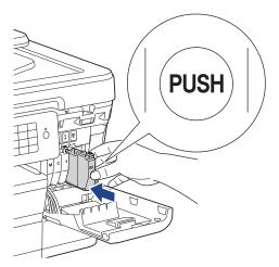
The machine will automatically reset the ink dot counter.
