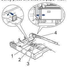
4. Load up to 20 sheets of photo paper in the paper tray with the printing surface *face down*. Loading more than 20 sheets of photo paper may cause paper jams.
