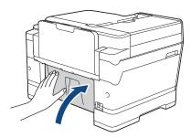
9. If your LCD error message was <code>[Jam Front/MP Tray]</code> or <code>[Repeat Jam Front/MP Tray]</code>, make sure you look carefully inside the MP tray for jammed paper. Push the release lever (1) towards the back of the machine, and then slowly pull the jammed paper out of the MP tray.
