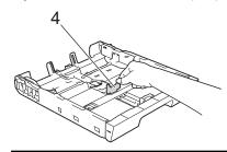
4. Fan the stack of paper well to avoid paper jams and misfeeds.
