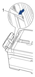
10. If your LCD error message was [Jam Front/Manual Feed Slot] or [Repeat Jam Front/Manual Feed], make sure you look carefully inside the manual feed slot for jammed paper and slowly pull it out of the machine.
