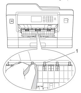
6. Lift the Jam Clear Flap (2), and then clean the back side of the Paper Feed Rollers (1) with a soft lint-free cloth moistened with water. After cleaning, wipe the rollers with a dry, soft lint-free cloth to remove all moisture.
