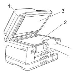
3. In the ADF unit, clean the white bar (1) and the glass strip (2) with a lint-free cloth moistened with water.
