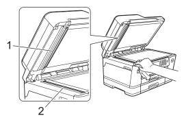
4. (MFC-J3930DW/MFC-J6930DW/MFC-J6935DW) Open the scanner glass cover (1), and clean the white bar (2) and the glass strip (3) with a soft lint-free cloth moistened with water.
