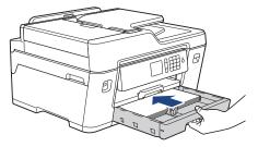
(MFC-J3930DW/MFC-J6930DW/MFC-J6935DW) Slowly push Tray #1 and Tray #2 (if removed) completely into the machine.
