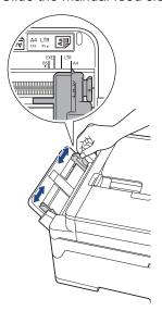
3. Load only one sheet of paper in the manual feed slot with the printing surface face up.
