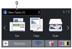
When [Fax Preview] is set to [On], [New Faxes] displays how many new faxes you have received and stored in the memory.
