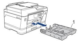
4. Lift the paper support (1), and then pull it at an angle completely out of the machine as shown by the arrow.
