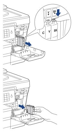
3. Open the new ink cartridge bag for the colour indicated on the LCD, and take out the ink cartridge.
