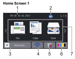
This screen shows the machine's status when the machine is idle. This Home screen is also called the Ready Mode screen. When displayed, it indicates that your machine is ready for the next command.
