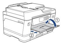
2. Pull the paper tray completely out of the machine as shown by the arrow.
