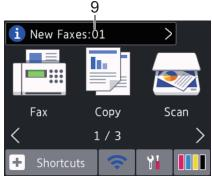
When [Fax Preview] is set to [On], [New Faxes] displays how many new faxes you have received and stored in the memory.
