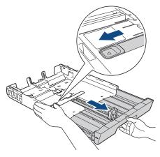
4. Gently press and slide the paper width guides (1) and then the paper length guide (2) to fit the paper size. Make sure the triangular mark (3) on the paper width guide (1) and paper length guide (2) line up with the marks for the paper you are using.
