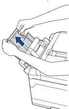
2. Gently press and slide the MP tray paper guides to match the width of the paper you are using.
