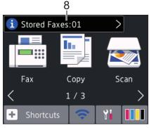
[Stored Faxes] displays how many received faxes are in the machine's memory.
