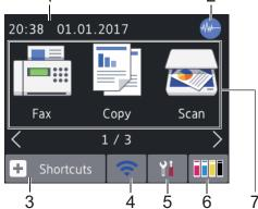
This screen shows the machine's status when the machine is idle. This Home screen is also called the Ready Mode screen. When displayed, it indicates that your machine is ready for the next command.
