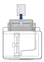
When loading an envelope, or a sheet of thick paper, push the envelope into the manual feed slot until
