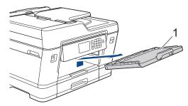
5. Clean the Paper Pick-up Rollers (1) with a soft lint-free cloth moistened with water. Slowly turn the rollers so that the whole surface is cleaned. After cleaning, wipe the rollers with a dry, soft lint-free cloth to remove all moisture.
