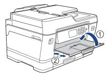
2. Pull the paper tray completely out of the machine as shown by the arrow.
