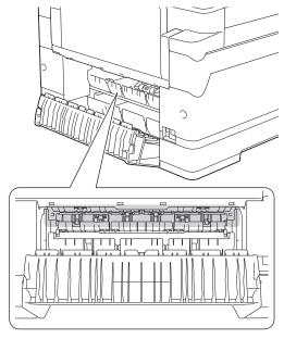
c. Close the Jam Clear Cover. Make sure the cover is closed completely.
