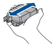
4. Insert the ink cartridge in the direction of the arrow on the label. Each colour has its own correct position.
