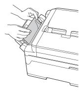
7. Using both hands, use the finger holds on each side of the machine to lift the scanner cover (1) into the open position.
