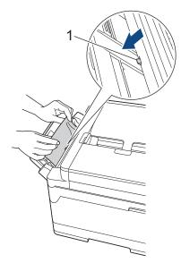
6. If your LCD error message was [Jam Manual Feed Slot] or [Repeat Jam Manual Feed Slot], slowly pull the jammed paper out of the manual feed slot.
