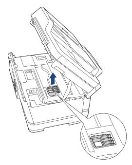
5. Gently close the scanner cover using the finger holds on each side.
