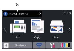
[Stored Faxes] displays how many received faxes are in the machine's memory.
