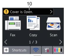
The warning icon • appears when there is an error or maintenance message; press • to view the details, and then press to return to Ready mode.
