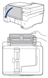
2. Slide the manual feed slot paper guides to fit the width of the paper you are using.
