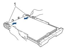
9. Make sure the paper is flat in the tray and below the maximum paper mark (1). Overfilling the paper tray may cause paper jams.
