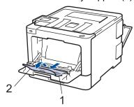
4. Slide the MP tray paper guides to fit the width of the paper that you are using. If the paper guide on the right side has a lever, press it and slide the paper guide.
