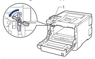
7. Gently slide the drum unit into the machine until it stops at the green lock lever.
