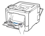
5. Load paper with the printing surface face up in the MP tray.
