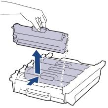
9. Turn the drum unit over by holding the green handles. Make sure that the drum unit gears (1) are on the left side.
