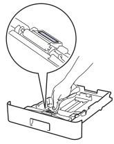
5. Wipe the two pick-up rollers inside the machine to remove dust.
