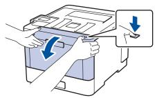
6. Hold the drum unit's green handle. Pull the drum unit out of the machine until it stops.
