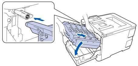
8. Turn the green lock lever clockwise to the lock position.
