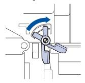
13. Using the green handle, push the drum unit back into the machine until it locks in place.
