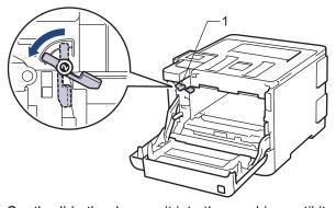
11. Gently slide the drum unit into the machine until it stops at the green lock lever.
