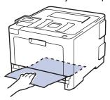
4. If paper is not jammed inside the machine, remove the paper from the paper tray, flip it over, and check underneath the paper tray.
