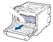
4. Turn the green lock lever (1) counterclockwise until it locks in the release position. Holding the green handles of the drum unit, lift the front of the drum unit and remove it from the machine.
