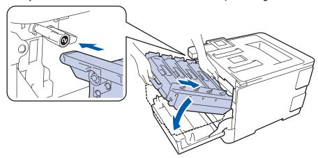
17. Turn the green lock lever clockwise to the lock position.
