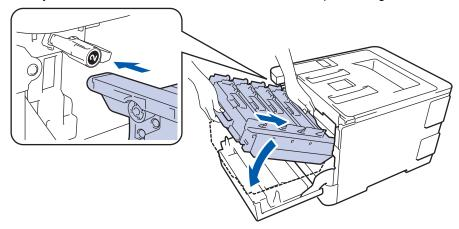
16. Turn the green lock lever clockwise to the lock position.
