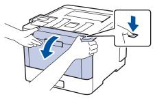
2. Hold the drum unit's green handle. Pull the drum unit out of the machine until it stops.
