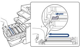
Replace the toner cartridge that matches the colour of the streak or band.
