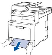
Pulling the jammed paper downward using both hands allows you to remove the paper more easily.
