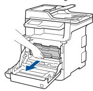
4. Hold the handle of the toner cartridge and gently push it away from you to unlock it. Pull it up and out of the drum unit. Repeat this for all toner cartridges.
