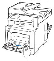
6. Load paper with the printing surface face up in the MP tray.
