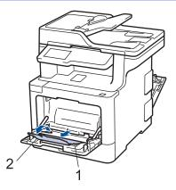
5. Slide the MP tray paper guides to fit the width of the envelopes that you are using.
