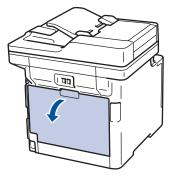
3. Pull the green levers at the left and right sides toward you to release the fuser cover.
