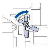
8. Using the green handle, push the drum unit back into the machine until it locks in place.
