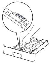
5. Wipe the two pick-up rollers inside the machine to remove dust.
