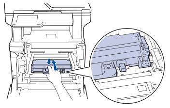
9. Slide the belt unit back into the machine. Make sure the belt unit is level and fits firmly into place.
