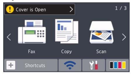
The warning icon \_\_\_\_ appears when there is an error or maintenance message. Press the message area to view it, and then press \_\_\_\_ to return to the Main Home screen.
