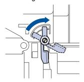
9. Using the green handle, push the drum unit back into the machine until it locks in place.
