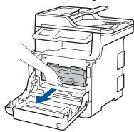
4. Turn the green lock lever (1) counterclockwise until it locks in the release position. Holding the green handles of the drum unit, lift the front of the drum unit and remove it from the machine.
