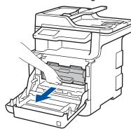
3. Turn the green lock lever (1) counterclockwise until it locks in the release position. Holding the green handles of the drum unit, lift the front of the drum unit and remove it from the machine.
