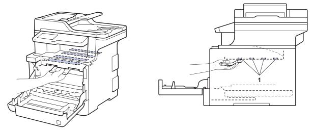
6. Make sure the green lock lever (1) is in the release position, as shown in the illustration.
