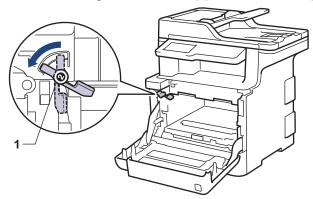
16. Gently slide the drum unit into the machine until it stops at the green lock lever.
