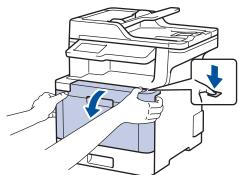
3. Hold the drum unit's green handle. Pull the drum unit out of the machine until it stops.
