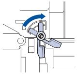
18. Using the green handle, push the drum unit back into the machine until it locks in place.
