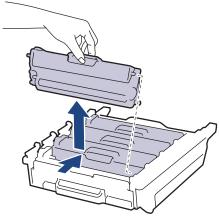
8. Reinsert the toner cartridge into the new drum unit and gently pull it toward you until you hear it lock into place. Make sure that you match the toner cartridge colour to the same colour label on the drum unit. Repeat this for all toner cartridges.
