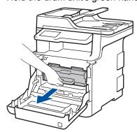
7. Turn the green lock lever (1) counterclockwise until it locks in the release position. Holding the green handles of the drum unit, lift the front of the drum unit and remove it from the machine.
