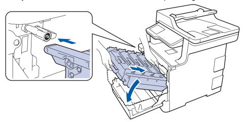
8. Turn the green lock lever clockwise to the lock position.
