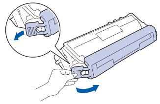
8. Insert the toner cartridge into the drum unit and gently pull it toward you until you hear it lock into place. Make sure that you match the toner cartridge colour to the same colour label on the drum unit. Repeat this for all toner cartridges.
