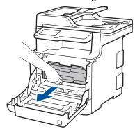
3. Hold the handle of the toner cartridge and gently push it away from you to unlock it. Pull it up and out of the drum unit. Repeat this for all toner cartridges.
