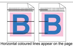
Identify the colour causing the problem and replace the toner cartridge that matches the colour of the line.
