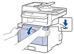
6. Hold the drum unit's green handle. Pull the drum unit out of the machine until it stops.
