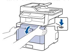
2. Hold the drum unit's green handle. Pull the drum unit out of the machine until it stops.
