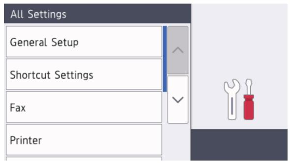
4. Swipe up or down or press ▲ or ▼ to display the [LCD Settings] option, and then press [LCD Settings].
