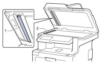
4. Open the scanner glass cover (1), and then clean the other white bar (2) and scanner glass strip (3) (supported models only).
