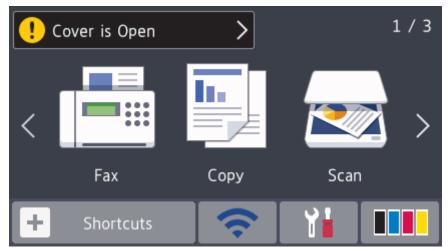
The warning icon \_\_\_\_ appears when there is an error or maintenance message. Press the message area to view it, and then press \_\_\_\_ to return to the Main Home screen.
