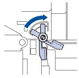
13. Using the green handle, push the drum unit back into the machine until it locks in place.
