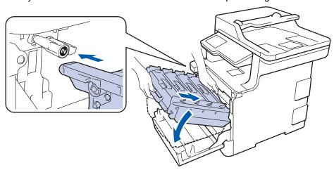
17. Turn the green lock lever clockwise to the lock position.
