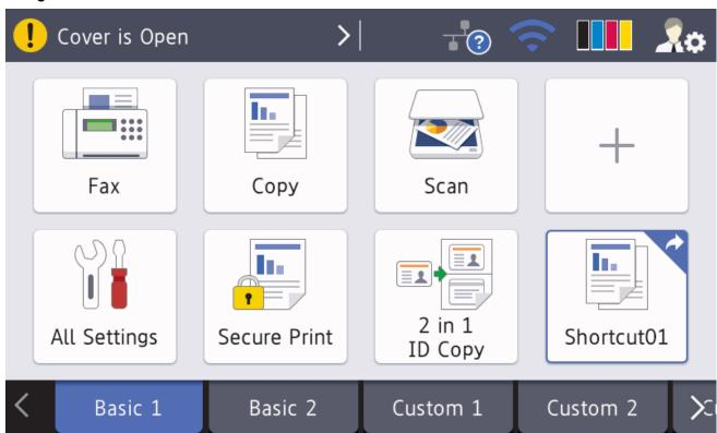
The warning icon \_\_\_\_ appears when there is an error or maintenance message. Press the message area to view it, and then press \_\_\_\_ to return to the Main Home screen.
