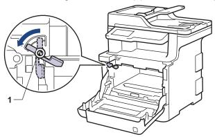
11. Gently slide the drum unit into the machine until it stops at the green lock lever.
