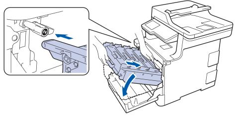
12. Turn the green lock lever clockwise to the lock position.
