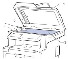
3. In the ADF unit, clean the white bar (1) and the scanner glass strip (2) underneath it with a soft lint-free cloth moistened with water.
