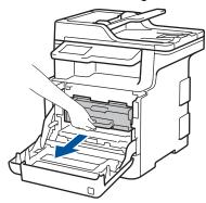
3. Hold the handle of the toner cartridge and gently push it away from you to unlock it. Pull it up and out of the drum unit. Repeat this for all toner cartridges.
