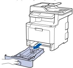
3. Make sure the jammed paper does not remain inside the machine.
