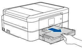
Pull the paper tray completely out of the machine.
