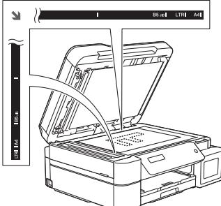
A line drawing of the DCP-T710W printer with its scanner glass open. An inset shows a document being placed on the glass. A vertical ruler on the left indicates the height of the document. The control panel is visible at the top right with settings like 'BS-A4', 'LTW', and 'A4'. <p>Placez le document face imprimée vers le bas dans le coin supérieur gauche de la vitre du scanner.</p> |
