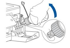
Remove the tip of the ink bottle. Insert the nozzle of the ink bottle firmly so that the ink does not spill. Fill the ink tank by gently squeezing the bottle as shown. Empty the entire bottle into the ink tank.
