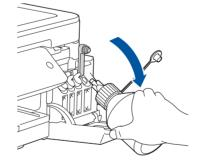
Point the nozzle upward so that the ink does not spill, and then remove the nozzle from the ink tank.
