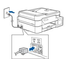
Connect the telephone line cord. Use the jack marked LINE.
