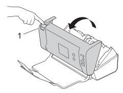
3. While pushing the right side of the Pick Up Roller Cover (1) from the front of the machine, pull the cover down.
