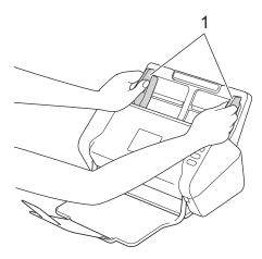
2. Place the card, *face down*, *top edge first* in the ADF between the Paper Guides until you feel it touch the inside of the machine.
