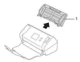
2. Press the release tab to open the Front Cover (1).
