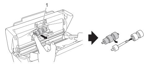
4. Fit the shaft of the new Brake Roller (1) into the slot in the opening and insert the Brake Roller into the machine.
