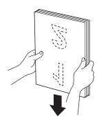
4. Place your document, *face down*, *top edge first* in the ADF between the Paper Guides until you feel it touch the inside of the machine. Feed thin pages slowly and carefully to keep the edge from being folded.
