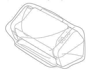
5. Pack the machine and the printed materials in the original carton with the original packing material as shown.
