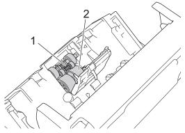
5. Fit the new lower Pick Up Roller into the opening, and then slide it to the left onto the shaft.
