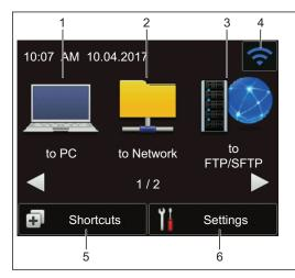
Home Screen 1 provides access to Scan to PC, Scan to Network, and Scan to FTP/SFTP operations.
