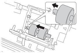
6. Fit the new upper Pick Up Roller into the opening, and then slide it to the left onto the shaft.
