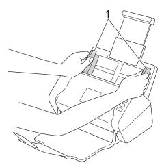
3. Place the Carrier Sheet, *face down* in the ADF between the Paper Guides until you feel it touch the inside of the machine.
