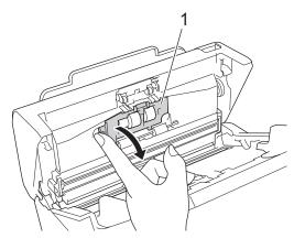
3. Lift the shaft of the Brake Roller (1) with your finger to remove the roller.
