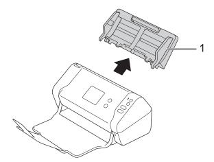
3. Press the release tab to open the Front Cover (1).
