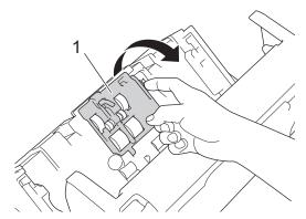
4. Slide the upper Pick Up Roller (1) to the right, and then pull it out to remove it. Remove the lower Pick Up Roller (2) in the same way.
