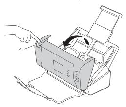
2. While pushing the left side of the Brake Roller Cover (1) from the back of the machine, pull the cover down.
