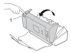
4. From the back of the machine, clean the glass strips in the ADF unit (1) with a soft lint-free cloth.
