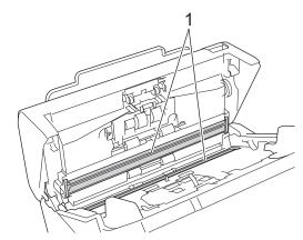
5. While pushing the left side of the Brake Roller Cover (1), pull the cover down.
