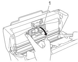
6. Lift the shaft of the Brake Roller (1) with your finger to remove the roller.
