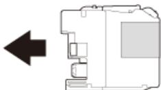
6. Gently push the area marked "PUSH" until the ink cartridge latches, and then close the ink cartridge cover.
