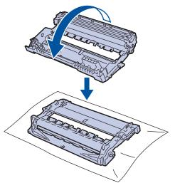
10. Use the numbered markers next to the drum roller to find the mark on the drum. For example, a dot in column 2 on the check sheet means that there is a mark in drum region "2".
