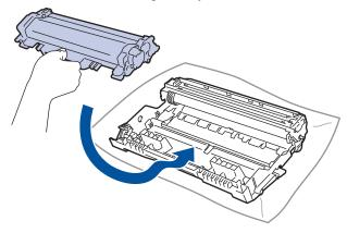
$^\prime$  Make sure you put the toner cartridge in correctly or it may separate from the drum unit.
