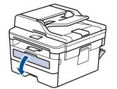
4. Use both hands to slide the manual feed slot paper guides to fit the width of the paper that you are using.
