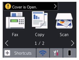
The warning icon ① appears when there is an error or maintenance message; press the message area to view it, and then press X to return to Ready Mode.
