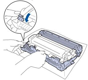
11. Turn the drum unit as shown in the illustration. Make sure that the drum unit gear is on the left side.
