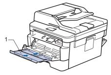
5. Slide the MP tray paper guides to fit the width of the envelopes that you are using.
