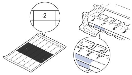
11. Turn the edge of the drum unit towards you while looking at the drum surface to find the mark.
