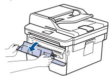
3. Remove the toner cartridge and drum unit assembly.
