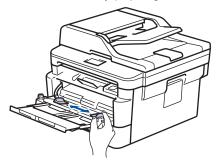
5. Load paper with the printing surface *face up* in the MP tray.
