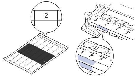
13. Turn the edge of the drum unit towards you while looking at the drum surface to find the mark.
