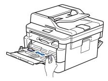
6. Load paper with the printing surface face up in the MP tray.
