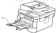
4. Slide the MP tray paper guides to fit the width of the paper you are using.
