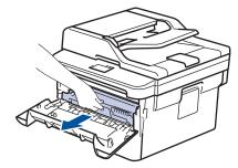
10. Push down the green lock lever and take the toner cartridge out of the drum unit.
