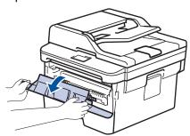
2. Remove the toner cartridge and drum unit assembly from the machine.
