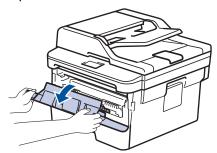
3. Remove the toner cartridge and drum unit assembly from the machine.
