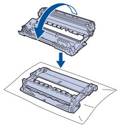
12. Use the numbered markers next to the drum roller to find the mark on the drum. For example, a dot in column 2 on the check sheet means that there is a mark in drum region "2".
