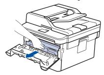
3. Clean the corona wire inside the drum unit by gently sliding the green tab from left to right and right to left several times.
