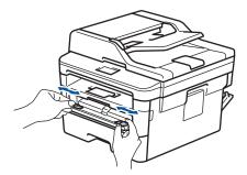
5. Using both hands, put one envelope in the manual feed slot until the front edge touches the paper feed roller. When you feel the machine pull it in, let go.
