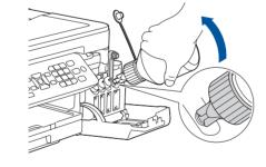
Insert the nozzle of the ink bottle firmly so that the ink does not spill. Fill the ink tank by gently squeezing the bottle as shown. Empty the entire bottle into the ink tank.
