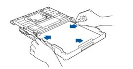
Adjust the paper guides. Fan the paper well and load it in the tray.
