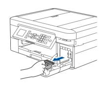
Open the ink cartridge cover, and then remove the orange protective part from the machine.
