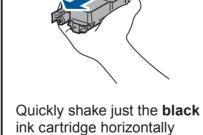
15 times as shown, before inserting it into the machine.
