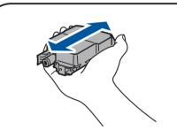
Quickly shake just the **black** ink cartridge horizontally 15 times as shown, before inserting it into the machine.
