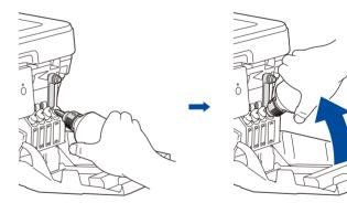
Remove the nozzle cap and insert the bottle nozzle firmly into the ink tank so that the ink does not spill.
