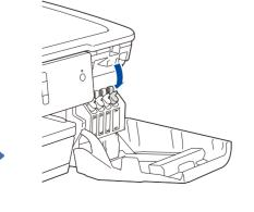
Push down on the cap of the ink tank to close it tightly. Repeat step 6 for the three other ink tanks.
