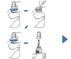
Remove the film and tighten the cap firmly.
