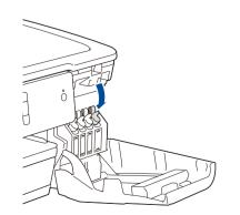
Push down on the cap of the ink tank to close it tightly. Repeat step 4 for the three other ink tanks.
