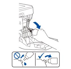
When finished, remove the bottle, pointing the nozzle upward so the ink does not spill.
