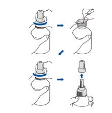
Remove the film and tighten the cap firmly.
