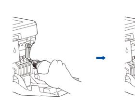
Remove the nozzle cap and insert the bottle nozzle firmly into the ink tank so that the ink does not spill.
