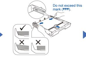
Adjust the paper guides. Fan the paper well and load it in the tray.
