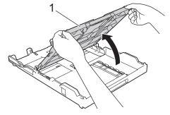
4. Load up to 10 envelopes in the paper tray with the printing surface **face down**. Loading more than 10 envelopes may cause paper jams.
