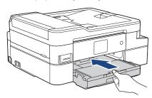
6. While holding the paper tray in the machine, pull out the paper support (1) until it locks into place, and then unfold the paper support flap (2).
