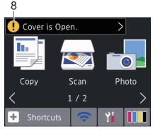
The warning icon \_\_\_\_ appears when there is an error or maintenance message; press \_\_\_\_ to view the details, and then press \_\_\_\_ to return to the Home screen.
