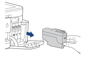
3. Open the new ink cartridge bag for the colour indicated on the LCD, and take out the ink cartridge.
