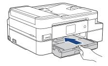
9. While holding the paper tray in the machine, pull out the paper support (1) until it locks into place, and then unfold the paper support flap (2).
