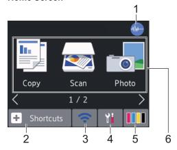
This screen shows the machine's status when the machine is idle. When displayed, it indicates that your machine is ready for the next command.
