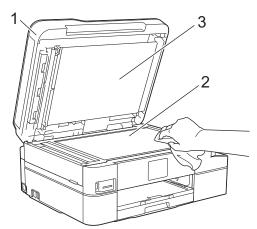
3. In the ADF unit, clean the white bar (1) and the glass strip (2) with a lint-free cloth moistened with water.
