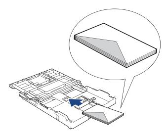
5. Gently press and slide the paper width guides (1) and paper length guide (2) to fit the size of the envelopes. Make sure the envelopes are flat in the tray.
